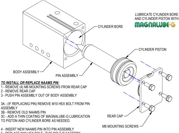
5 - REPLACE M10 HEX BOLT. THIS BOLT IS FACTORY SUPPLIED WITH VIBRA-TITE TO PREVENT THE SCREW FROM VIBRATING LOOSE.
